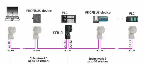
Fig. 6-1 Mini PROFIBUS Repeater PFB-R prolongs the communication distance and increases the stations.
