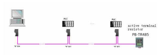
Fig. 7-2Active terminal resistor installed at the network terminal
