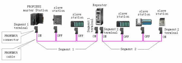
Fig.1-1 PROFIBUS fieldbus adopts bus network topological structure
