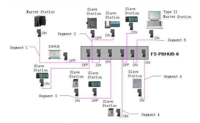
Fig. 2-1 Achieve PROFIBUS star and hybrid network topology structure by using hub
