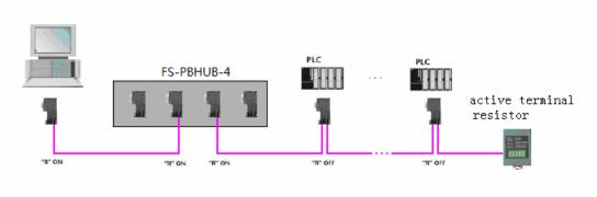
Fig. 7-2 Active Terminal Resistor Installed at the Network Terminal
