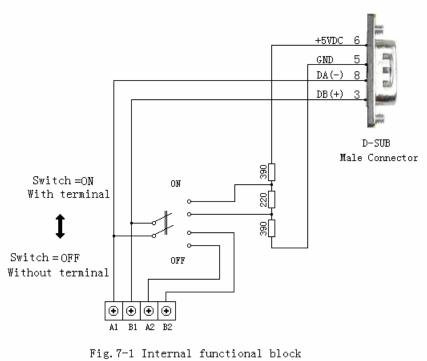
diagram of PROFIBUS bus connector plug
