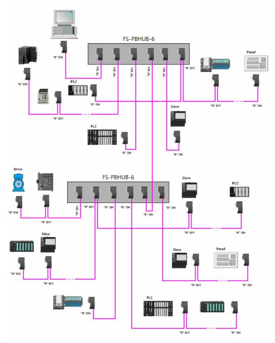
Fig. 6-3 Hybrid network topological structure through FS-PBHUB-6
