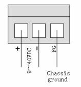
Wiring diagram of power terminal
