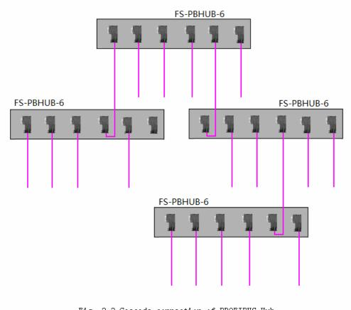
Fig. 2-2 Cascade connection of PROFIBUS Hub
